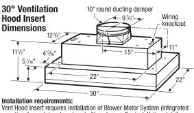
Vent Hood Insert requires installation of Blower Motor System (integrated or optional remote) and custom-built enclosure. For installation details and specifications, refer to Product installation Guide on web.
